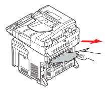
If the sheet is low down in this area and difficult to remove, it is probably still gripped by the fuser. In this case raise the top cover, reach around and press down on the fuser pressure release lever.
